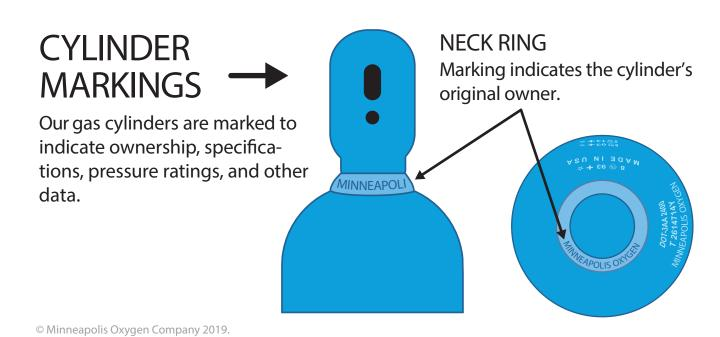
CYLINDER SPECIFICATION • Dept. of Transportation Specification Type of material of construction (3AA) • Service or working pressure in pounds per square inch (PSI) SERIAL NUMBER ~ POLIS OXYGE CYLINDER OWNER -OT-3AA2400 -2614714Y NEAPOLIS OXYGEN
